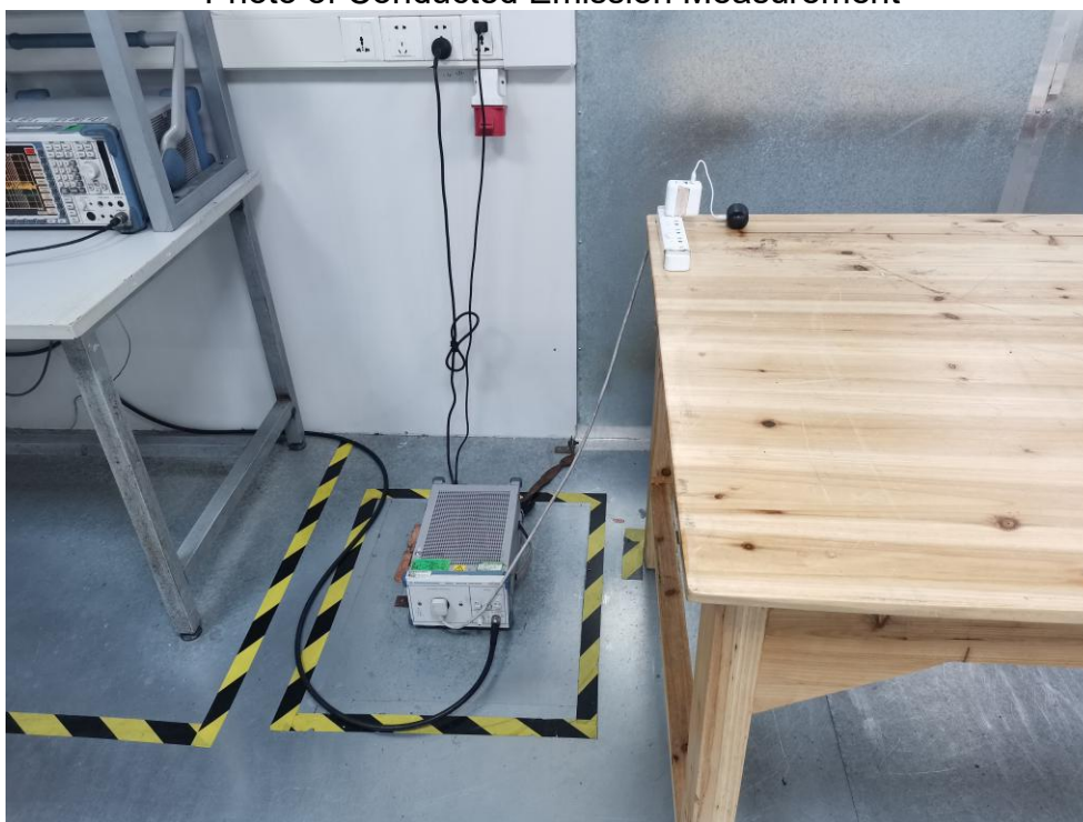
FCC ID: 2AJQ7CREW Photo of Conducted Emission Measurement
