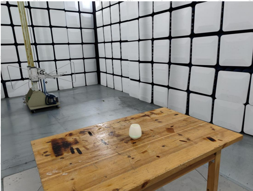
Photo of Radiation Emission Test
