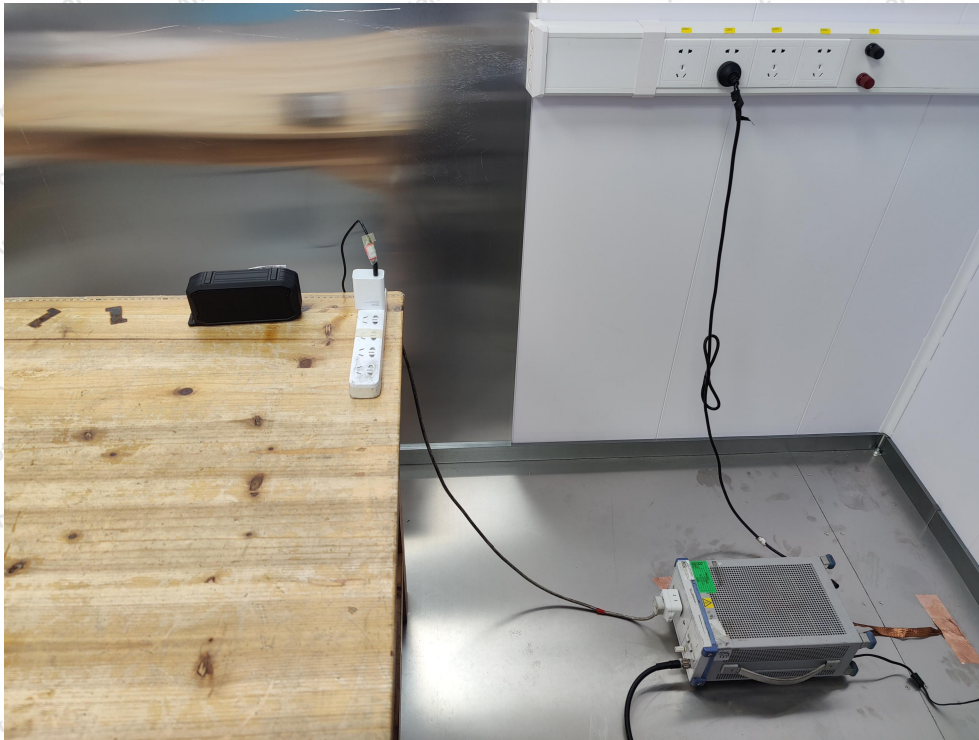
Photo of Conducted Emission Measurement
