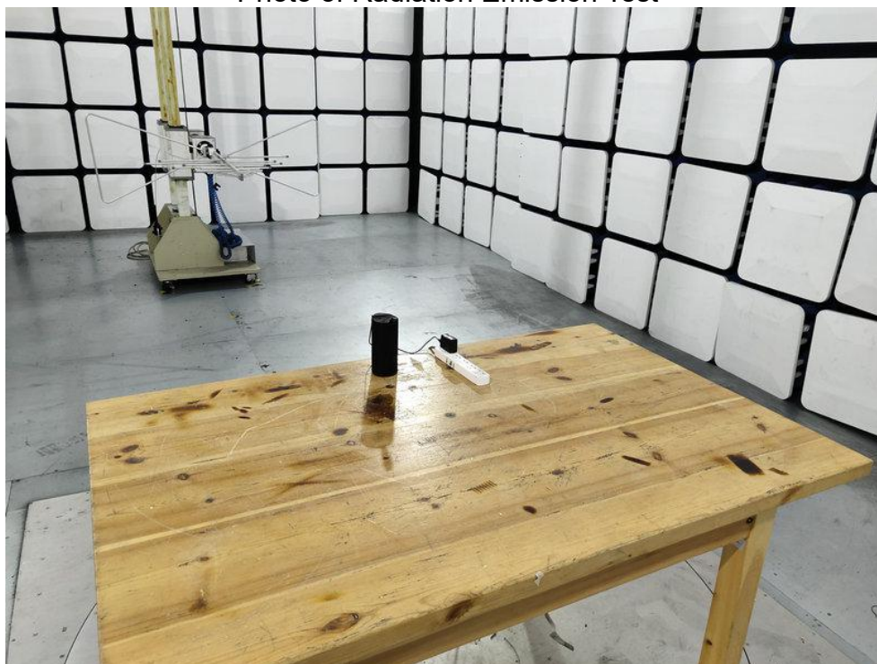
Photo of Radiation Emission Test
