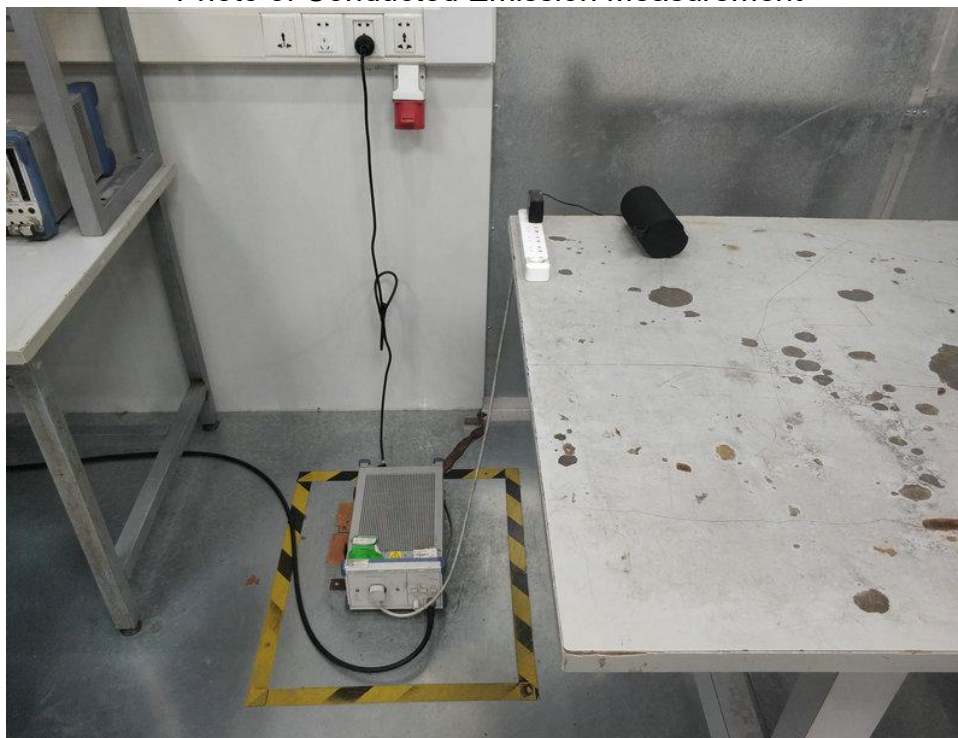
FCC ID:2AJQ7-IJRRSP01 Photo of Conducted Emission Measurement
