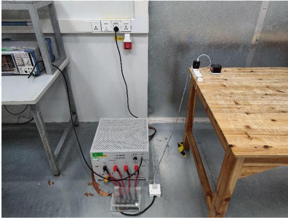
Photo of Conducted Emission Measurement
