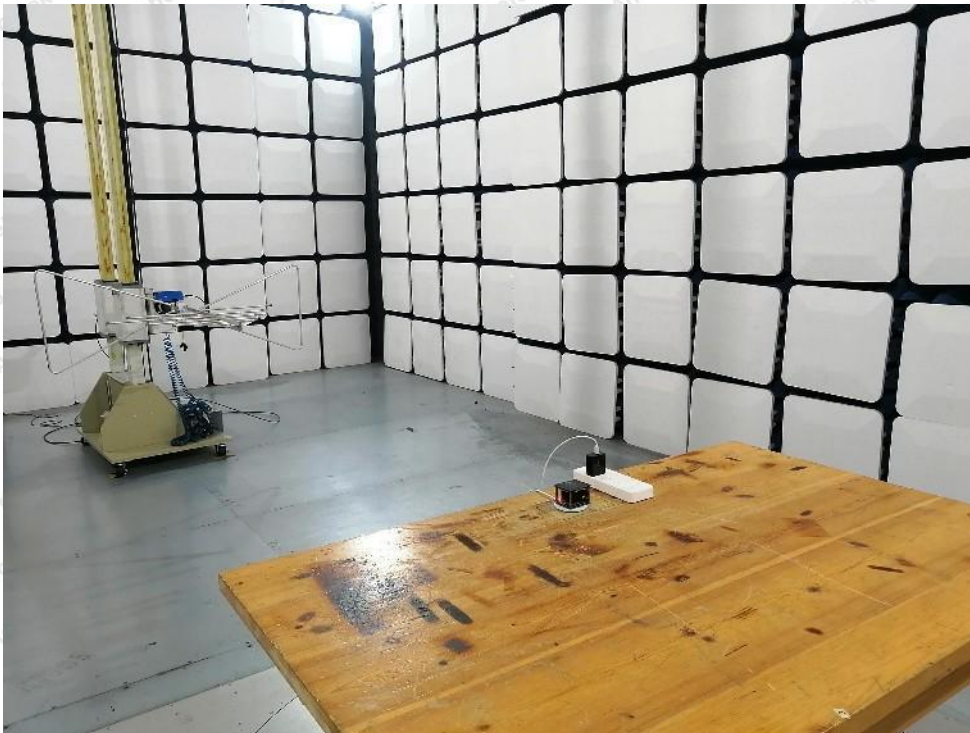
Photo of Radiation Emission Test
