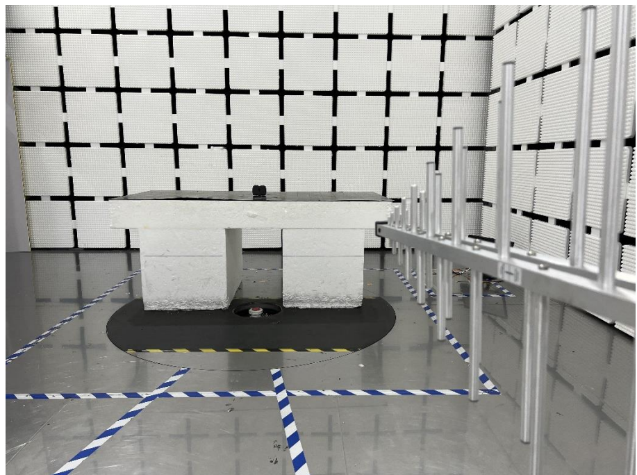
Radiation Emission Test Setup (30MHz to 1GHz)
