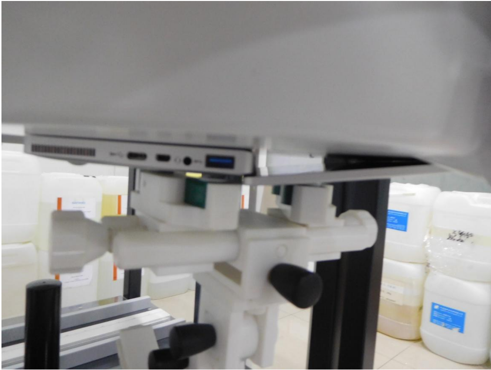
Flat front side-PAD (separation distance is 0mm)
