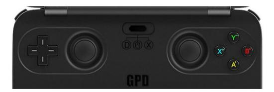
• Left joystick is taken as rolling button of mouse, to use to rolling up or down the
