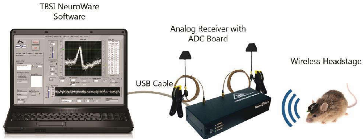
Figure 4: Standard TBSI Wireless Recording Setup
