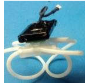
Figure 22: Rat Saddle Harness with Mounted 500 mAh External Battery
