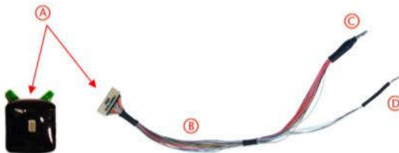
Figure 16: Headstage and Signal Transmission Test Cable
