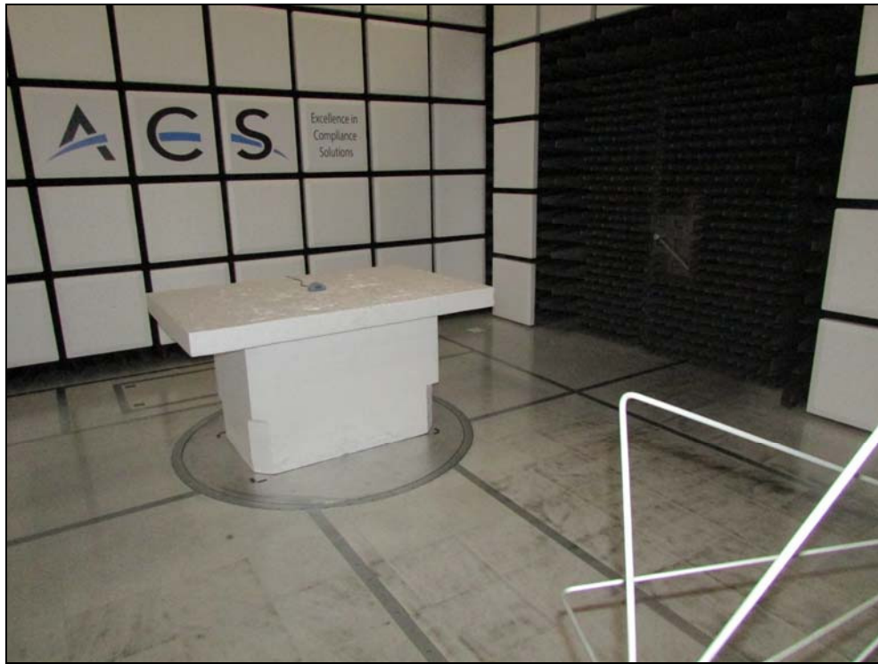
Figure 3: Radiated Emissions - Below 1GHz – Front View
