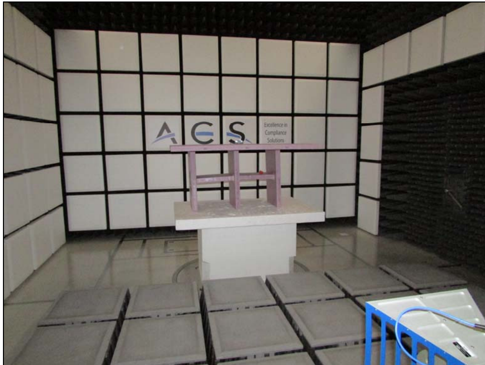
Figure 1: Radiated Emissions - Above 1GHz – Front View
