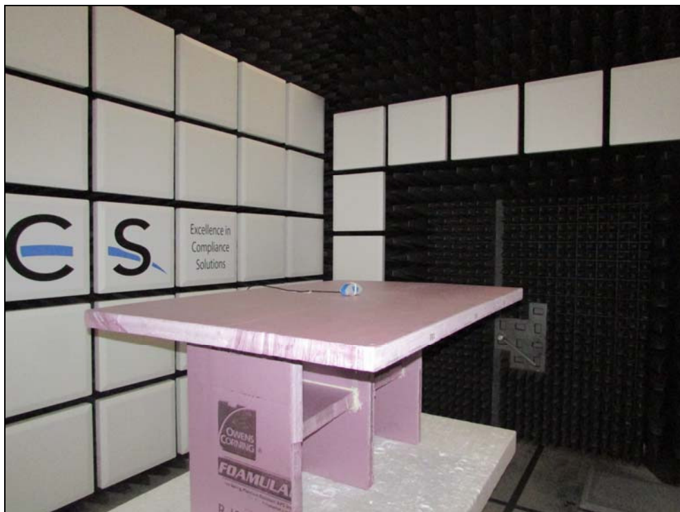
Figure 2: Radiated Emissions - Above 1GHz – Side View
