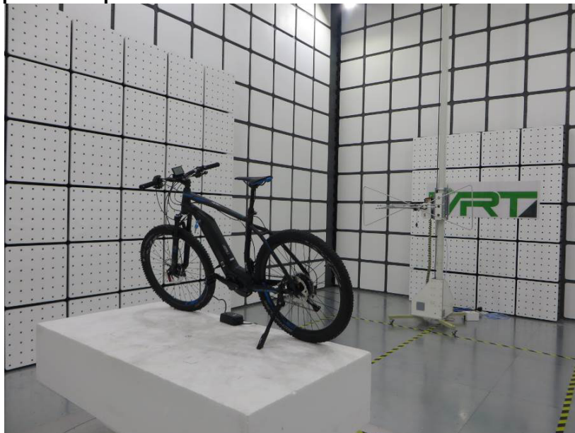
Photograph 2: Set-up for Radiated Test from 30MHz to 1GHz
