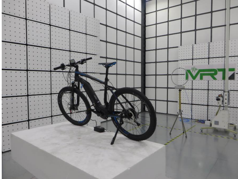
Photograph 1: Set-up for Radiated Test below 30MHz
