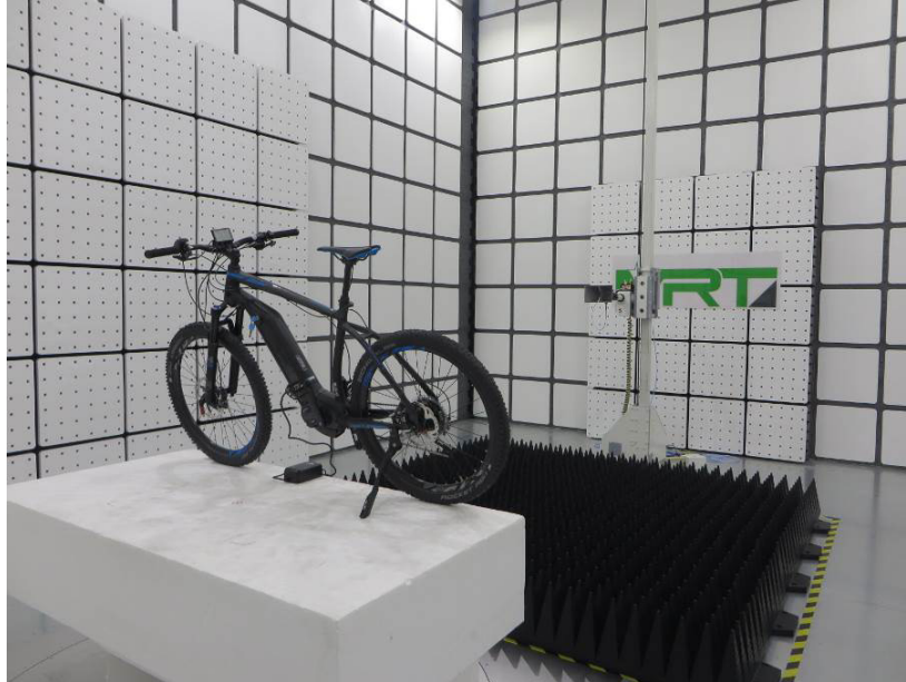
Photograph 3: Set-up for Radiated Test above 1GHz
