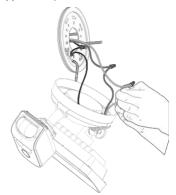
G. Carefully push all the wires through the large opening in the bracket. Align the mounting posts with the holes on floodlight cam and press together, securing the screw cap nuts with the screwdriver.
