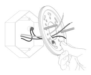
D. Make sure your existing wires come through the middle of the bracket. Attach the bracket to your junction box using at least two screws.
