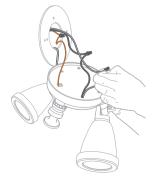
G. Carefully push all the wires through the large opening in the bracket. Align the mounting posts with the holes on floodlight cam and press together, securing the screw cap nuts with the orange screwdriver handle.
