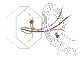
D. Make sure your existing wires come through the middle of the bracket. Attach the bracket to your junction box using at least two screws.
