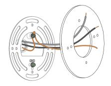
E. Use the provided hook to hang floodlight cam from the bracket while connecting the wires.
