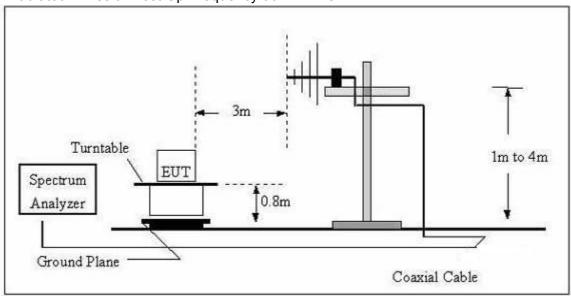
(C) Radiated Emission Test-Up Frequency Above 1GHz
