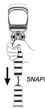
**TIP:** It's easier to snap them together if you place the bottom end on a firm surface and press down hard while holding the top. Press until you feel the "snap".
