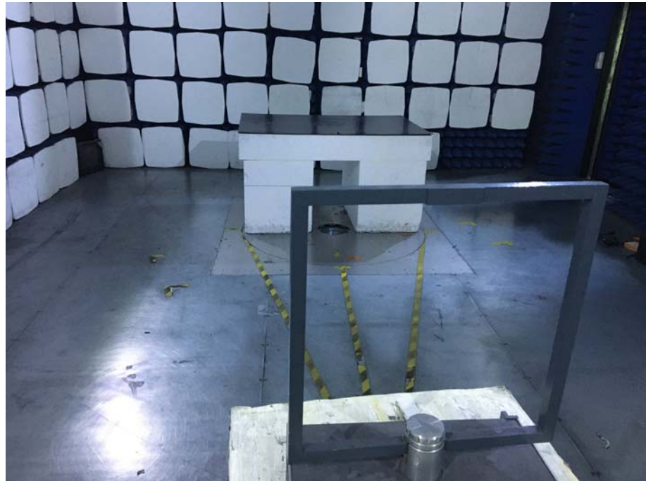
Radiation Emission Test Setup (Below 30MHz)
