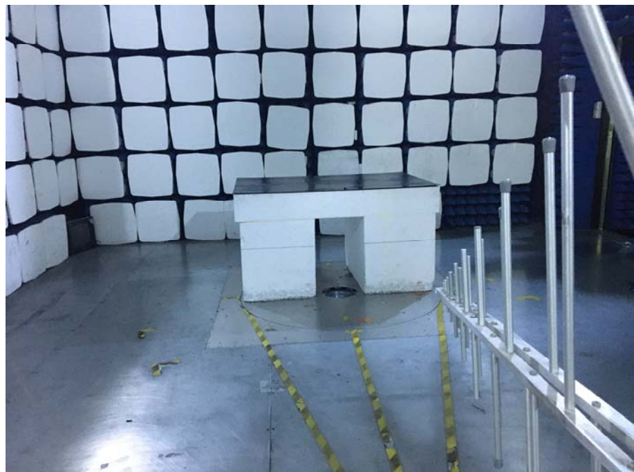
Radiation Emission Test Setup (30MHz to 1GHz)
