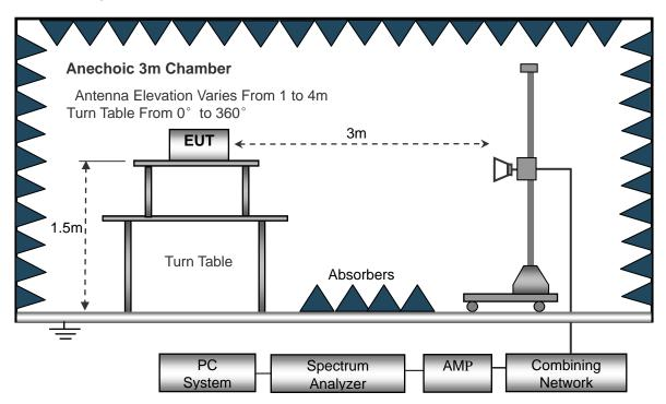
Frequency:9kHz-30MHz Frequency:30MHz-1GHz Frequency:Above 1GHz
