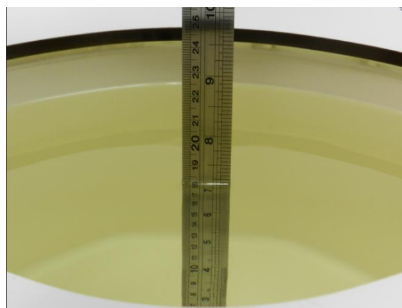
Fig 11.1.2 Photo of Liquid Height for Body SAR
