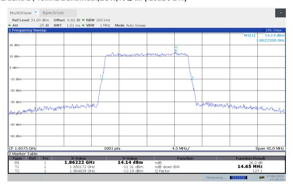
LTE band 2, 15MHz Bandwidth, HIGH, QPSK (-26dBc BW)
