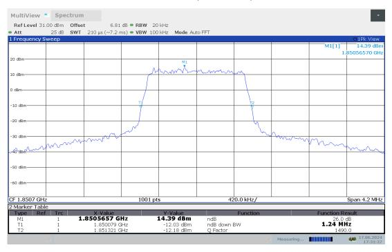
LTE band 2, 1.4MHz Bandwidth, HIGH, QPSK (-26dBc BW)
