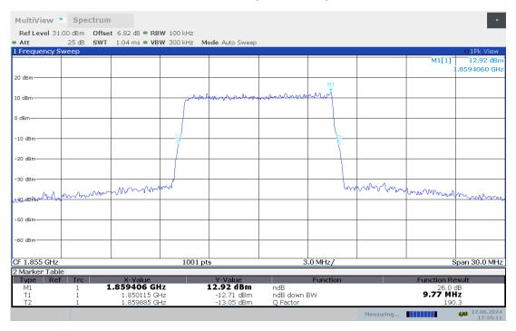
LTE band 2, 10MHz Bandwidth, HIGH, QPSK (-26dBc BW)
