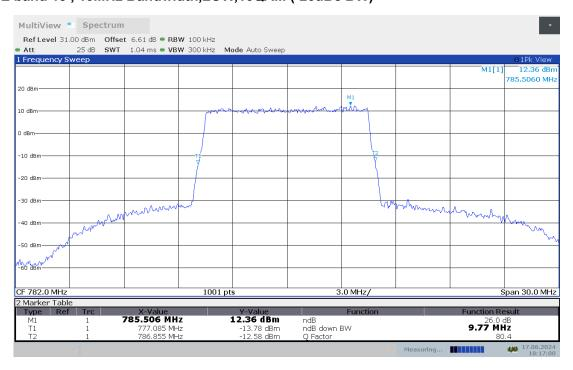
LTE band 13, 10MHz Bandwidth, HIGH, QPSK (-26dBc BW)
