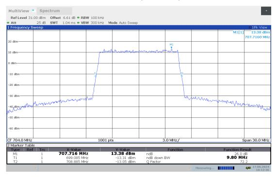
LTE band 12, 10MHz Bandwidth, HIGH, QPSK (-26dBc BW)
