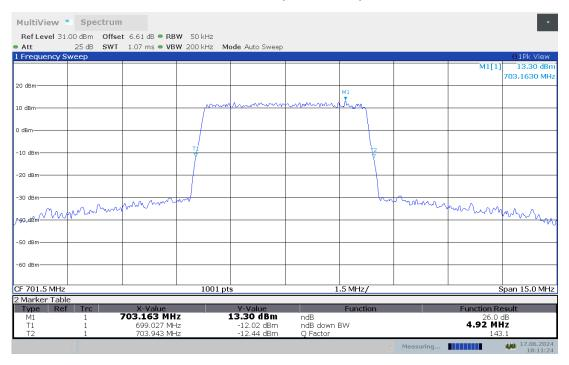
LTE band 12, 5MHz Bandwidth, HIGH, QPSK (-26dBc BW)
