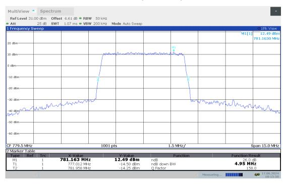
LTE band 13, 5MHz Bandwidth, HIGH, QPSK (-26dBc BW)
