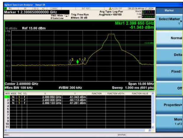
GFSK LOW CHANNEL, BAND EDGE
