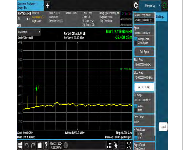
Band12 10MHz QPSK 23130 1RB#0 1000~10000 1000~10000
