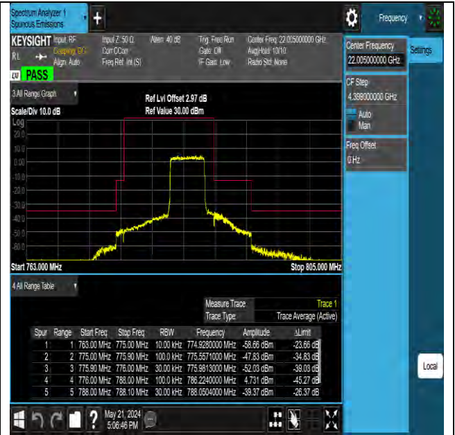
Band13 5MHz 16QAM 23255 25RB#0
