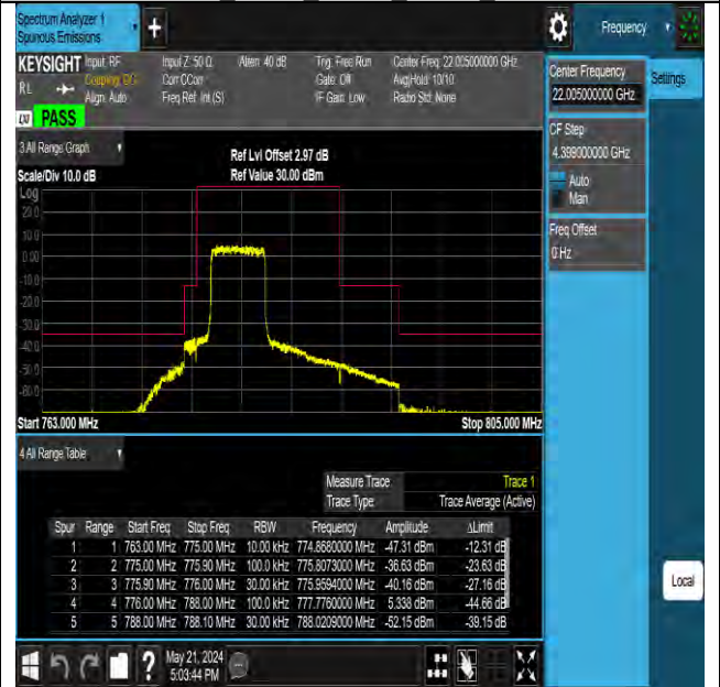
Band13 5MHz 16QAM 23205 25RB#0
