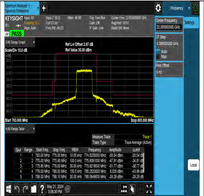
Band13 5MHz QPSK 23255 25RB#0
