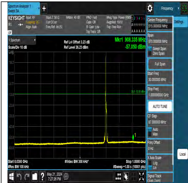
Band12 10MHz QPSK 23095 1RB#0 30~1000 30~1000
