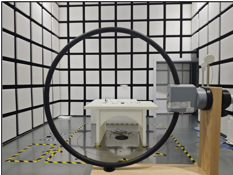
Fig. 1 Radiated emission setup photo(Below 30MHz)
