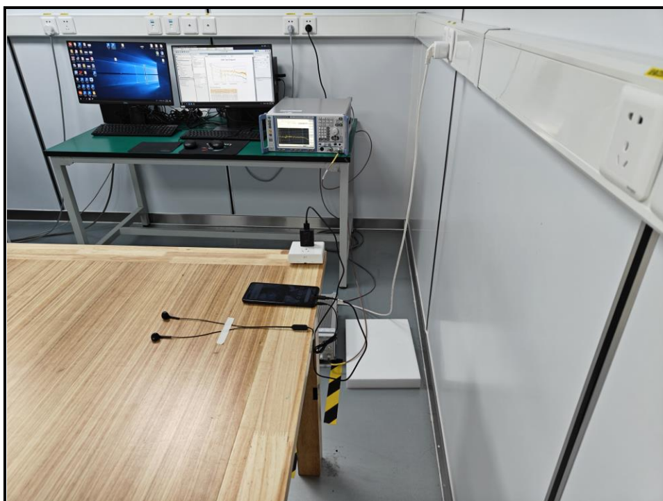
Fig. 4 Power line conducted emission setup photo
