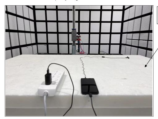
the absorbing material is under the foam
