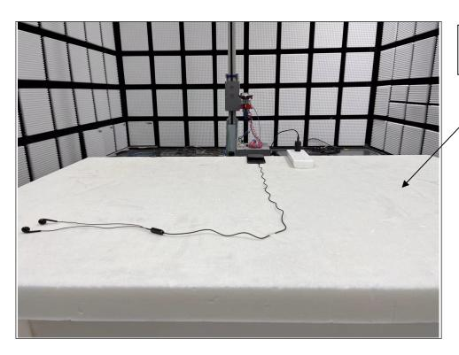
the absorbing material is under the foam
