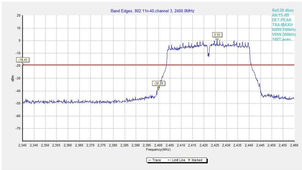
Fig.A.5.7 Band Edges (802.11n-HT40, Ch 3)
