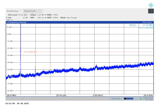
Note: The maximum value of expanded measurement uncertainty for this test item is U = 0.372 dB, k = 2.
