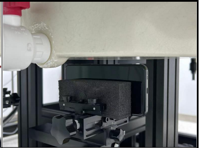
Right Side of EUT with 1.0 cm Gap
