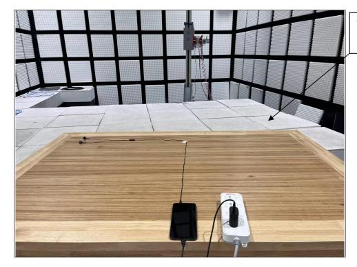
the absorbing material is under the foam
