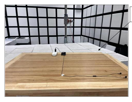
the absorbing material is under the foam
