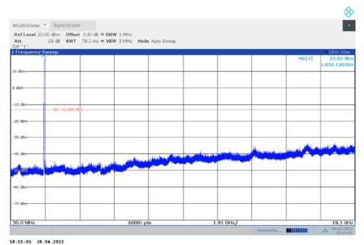
n5 NOTE: peak above the limit line is the carrier frequency.
