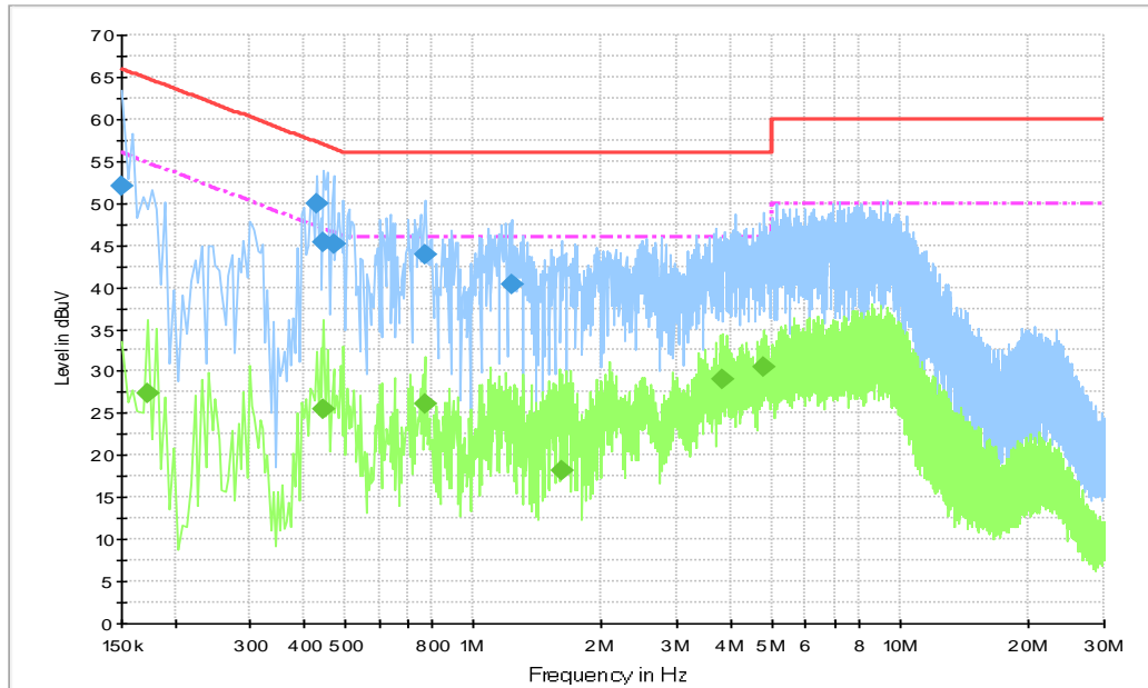
Fig. 23 AC Powerline Conducted Emission-Idle
