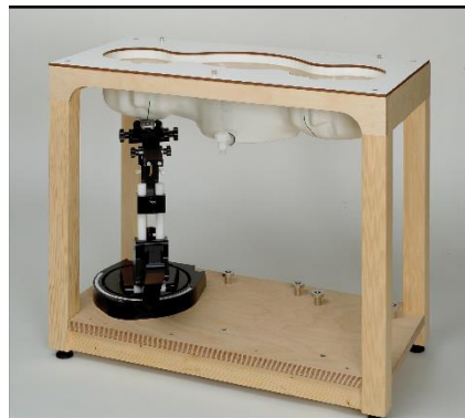
Picture C.10: SAM Twin Phantom
