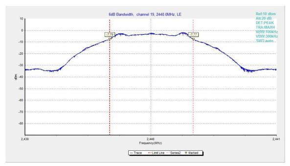
Fig.21. 6dB Bandwidth: GFSK, 2440 MHz
