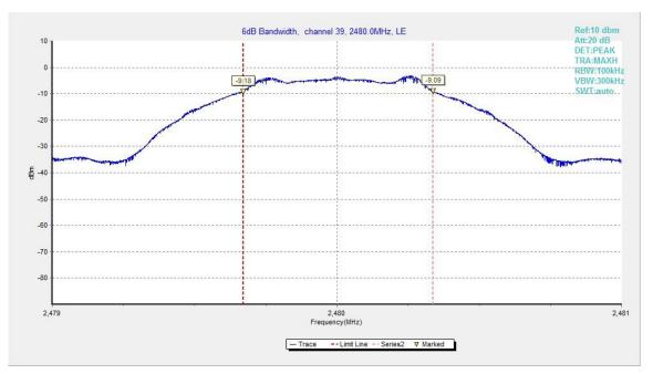
Fig.22. 6dB Bandwidth: GFSK, 2480 MHz
