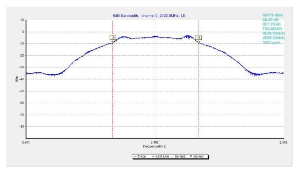
Fig.20. 6dB Bandwidth: GFSK, 2402 MHz
