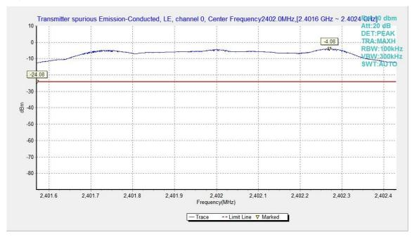
Fig.5. Transmitter Spurious Emission - Conducted: GFSK,2402MHz
