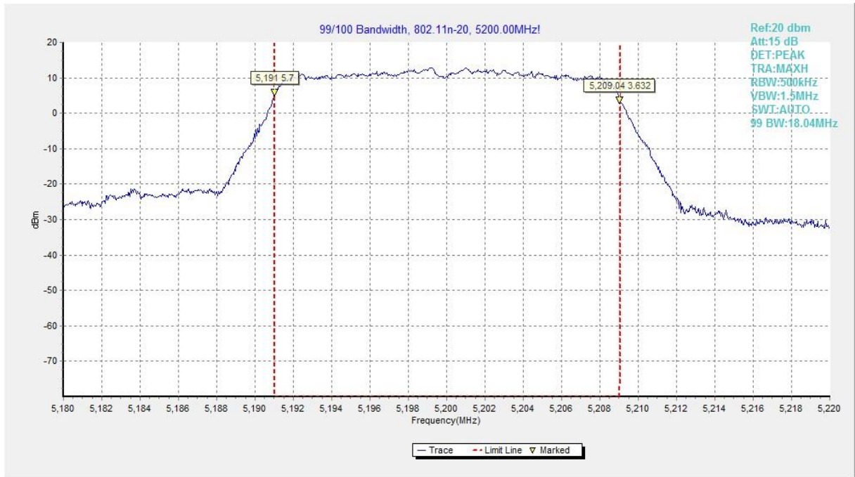
Fig.67 99% Occupied bandwidth (802.11n-HT20, 5200MHz)
