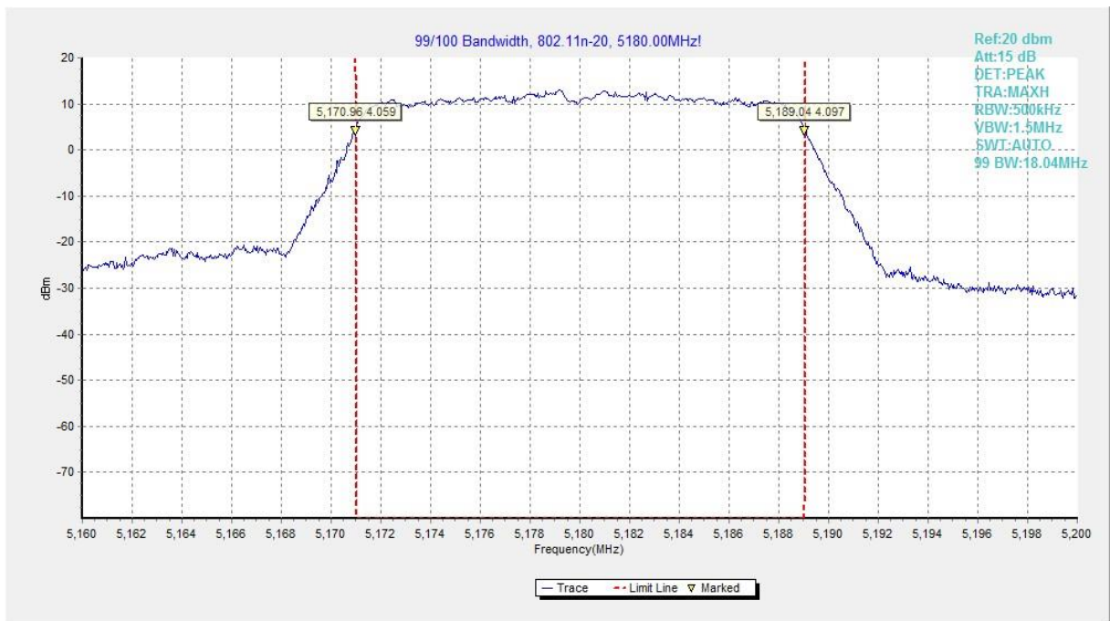
Fig.66 99% Occupied bandwidth (802.11n-HT20, 5180MHz)
