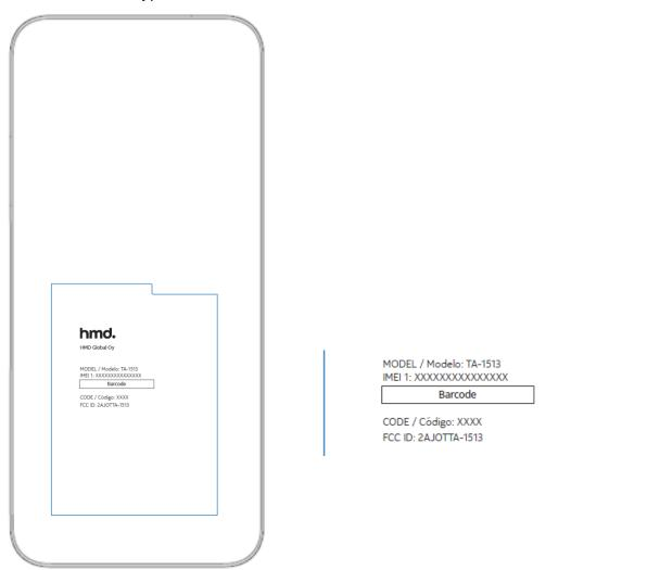
This device also has an electronic label for certification information. To access it, select Settings > System > Certification.
