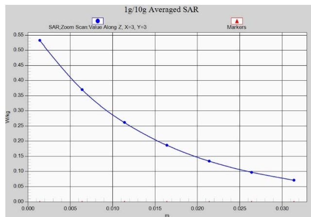
Fig. 1-18 Z-Scan at power reference point (LTE Band5)
