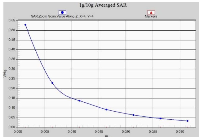
Fig. 1-15 Z-Scan at power reference point (LTE Band2)
