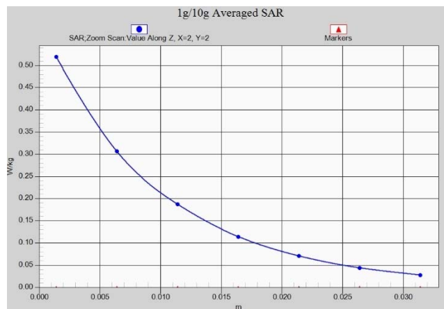
Fig. 1-9 Z-Scan at power reference point (WCDMA1700)
