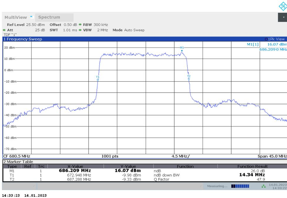
n71,15MHz Bandwidth,DFT-s-QPSK (-26dBc BW)
