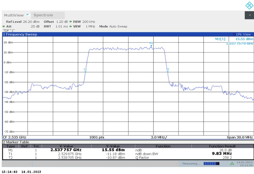
n7,10MHz Bandwidth,DFT-s-QPSK (-26dBc BW)
