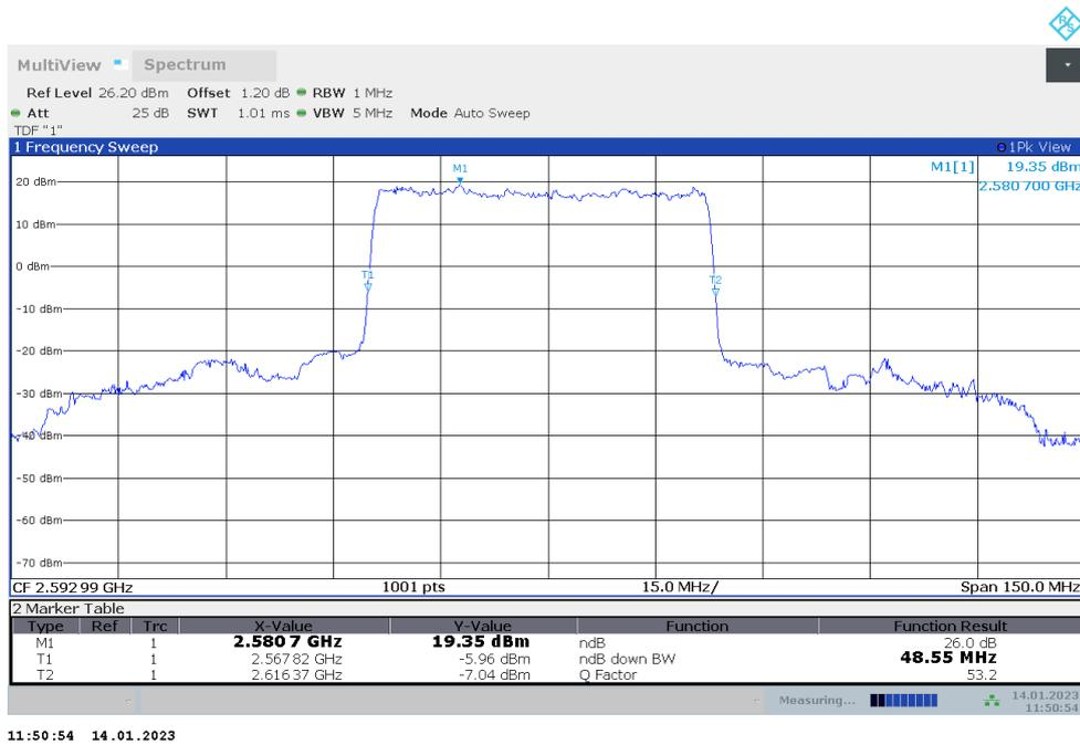
n41,50MHz Bandwidth,DFT-s-QPSK (-26dBc BW)
