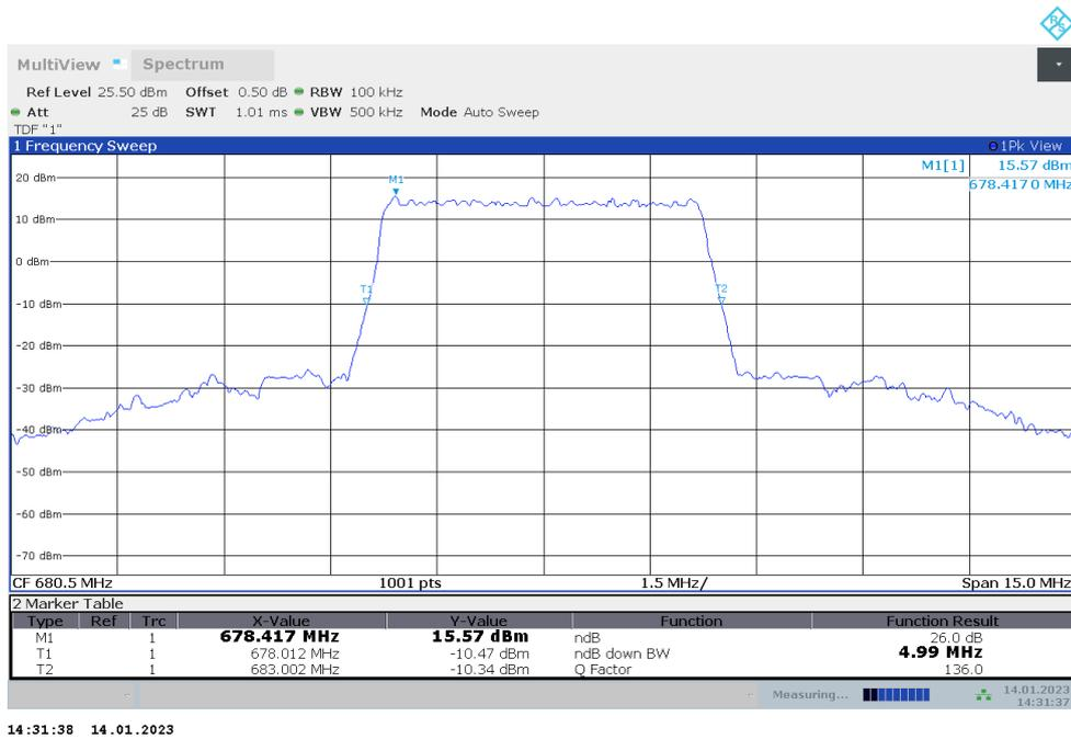
n71,5MHz Bandwidth,DFT-s-QPSK (-26dBc BW)
