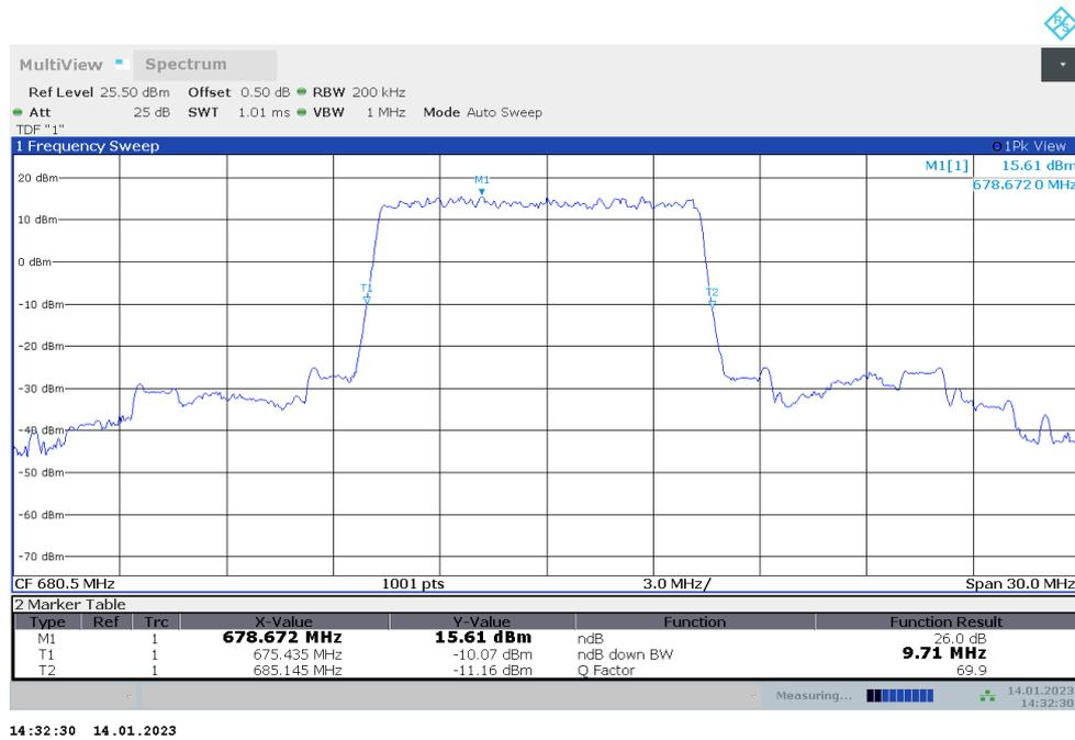
n71,10MHz Bandwidth,DFT-s-QPSK (-26dBc BW)
