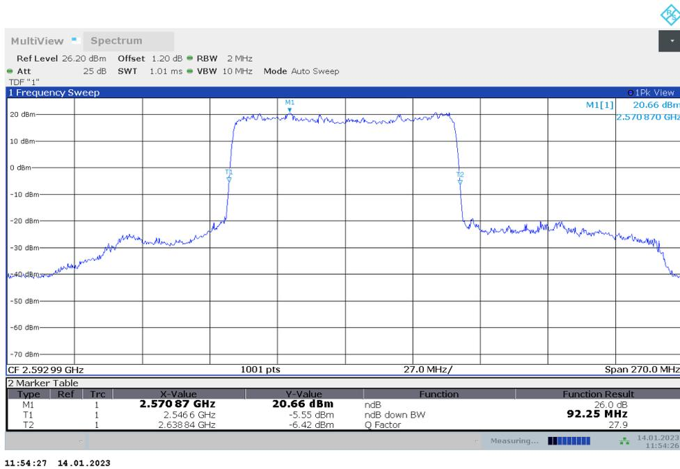
n41,90MHz Bandwidth,DFT-s-QPSK (-26dBc BW)
