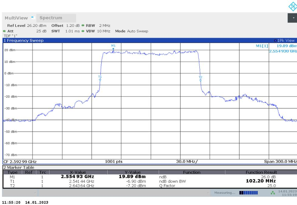
n41,100MHz Bandwidth,DFT-s-QPSK (-26dBc BW)
