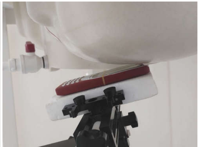
Left Tilted, Test Separation 0 mm
