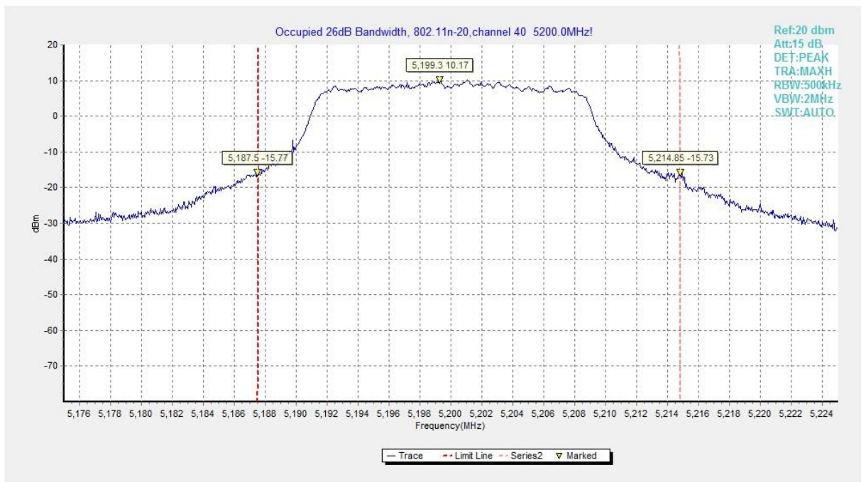
Fig.12 Occupied 26dB Bandwidth (802.11n-HT20, 5200MHz)
