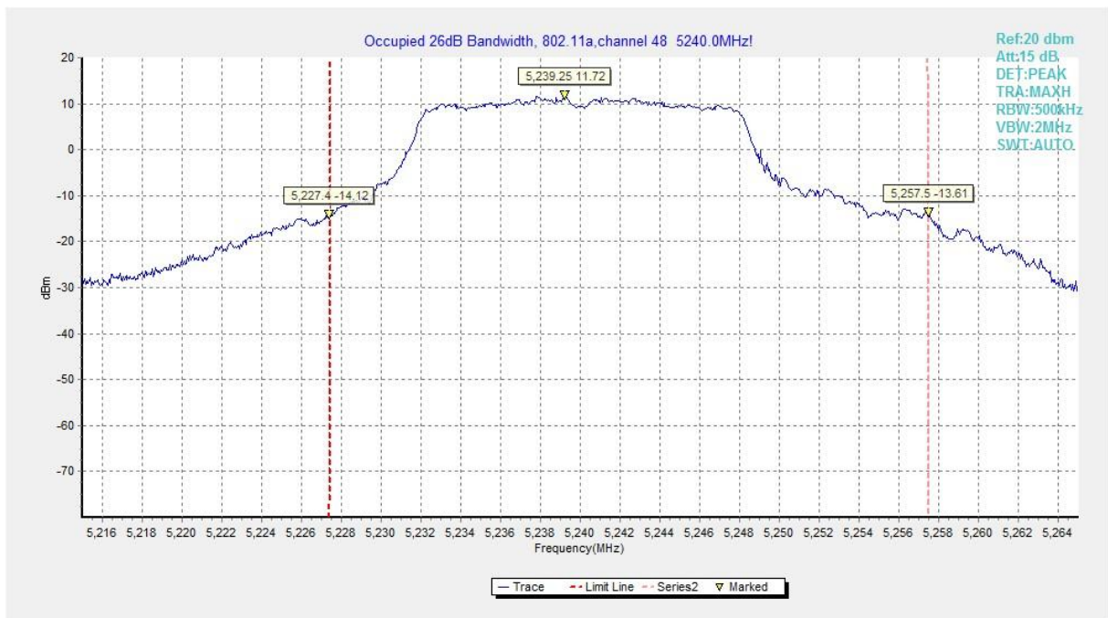
Fig.3 Occupied 26dB Bandwidth (802.11a, 5240MHz)
