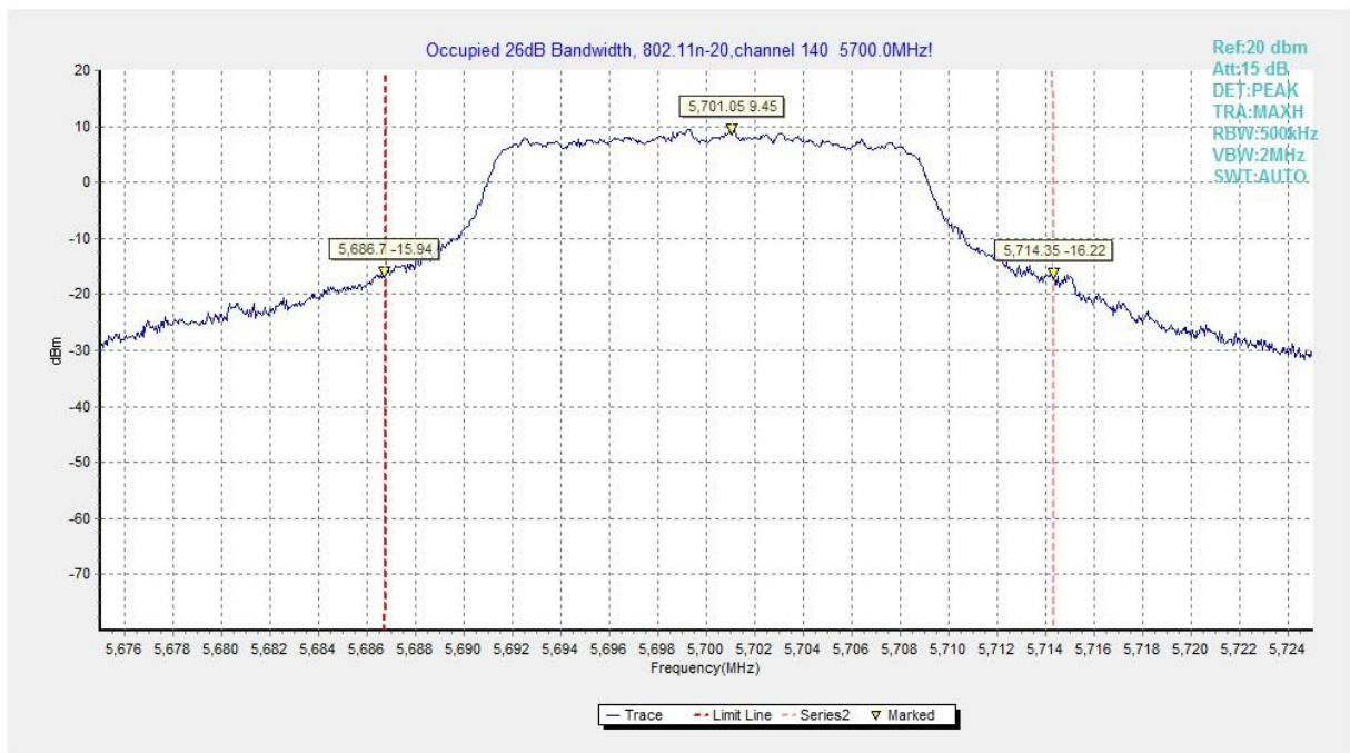
Fig.19 Occupied 26dB Bandwidth (802. 11n-HT20, 5700MHz)
