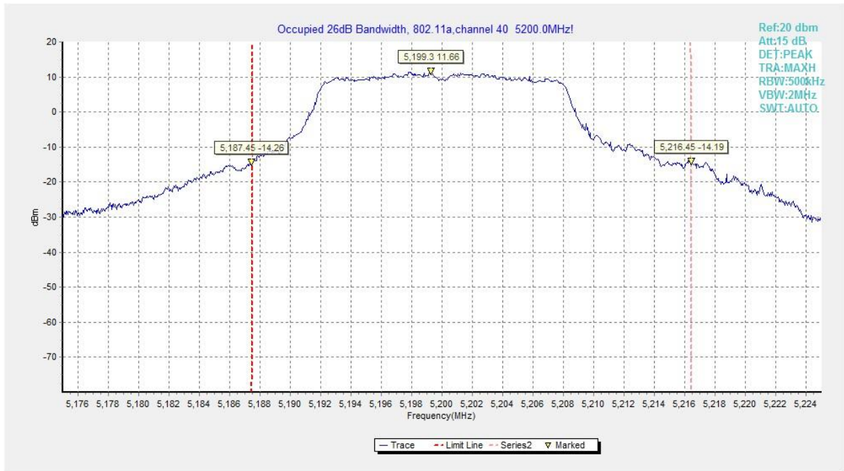
Fig.2 Occupied 26dB Bandwidth (802.11a, 5200MHz)
