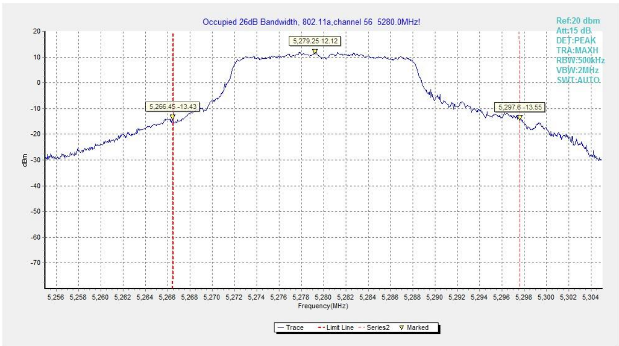
Fig.5 Occupied 26dB Bandwidth (802.11a, 5280MHz)
