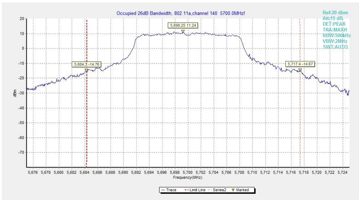
Fig.9 Occupied 26dB Bandwidth (802.11a, 5700MHz)
