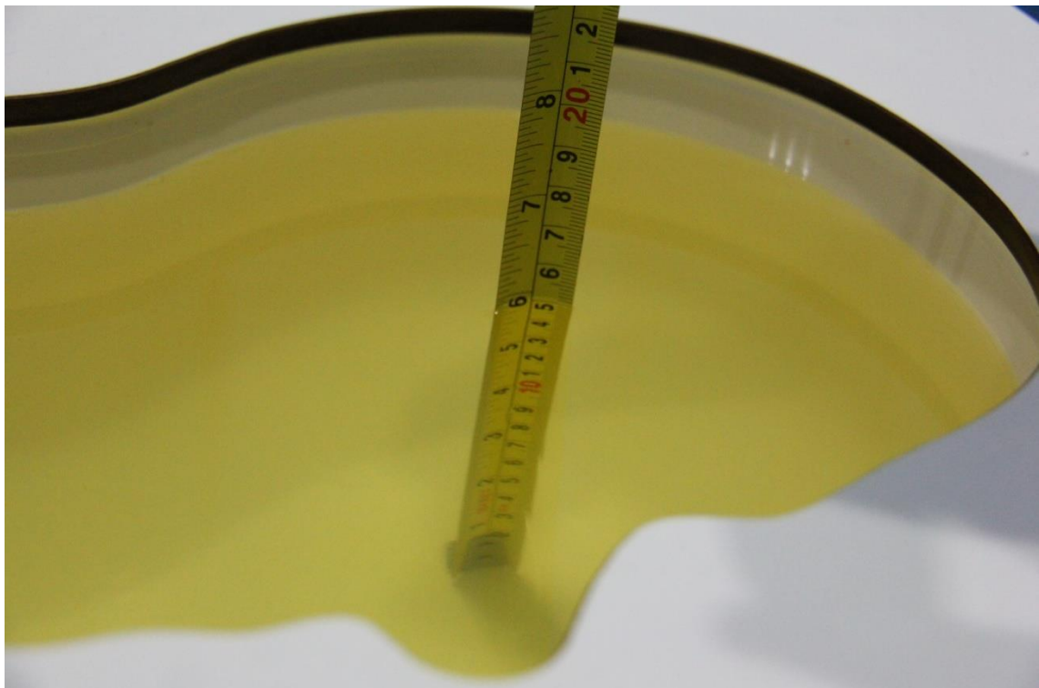
Picture 7-6 Liquid depth in the Head Phantom (3GHz)
