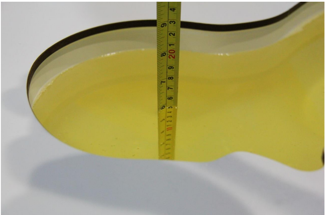
Picture 7-4 Liquid depth in the Head Phantom (2450MHz)
