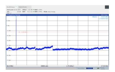
**Channel 1513: 30MHz –17.55GHz** Spurious emission limit –13dBm.
