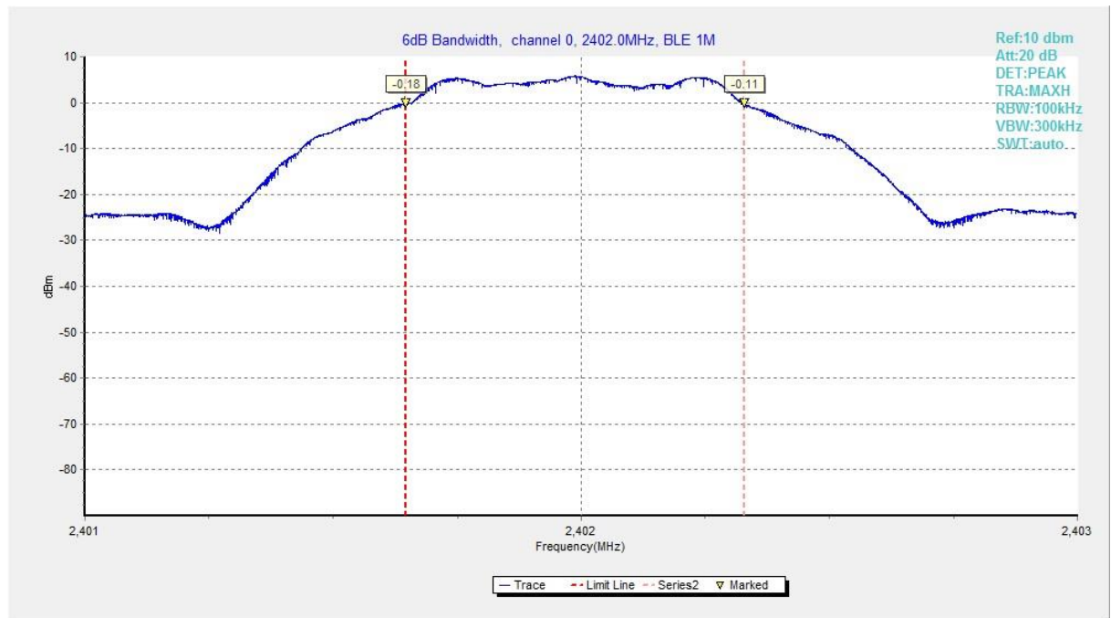
Fig.4 6dB Bandwidth (Ch 0), LE 1M
