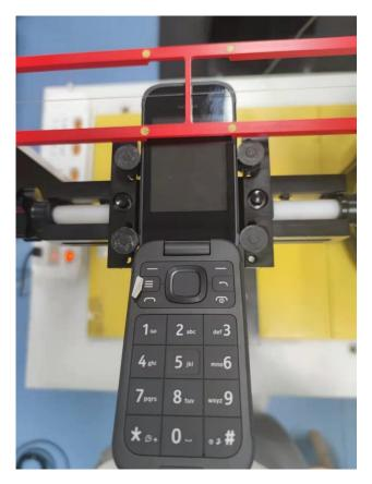
Picture 2: EUT Positioning for RF/T-coil
