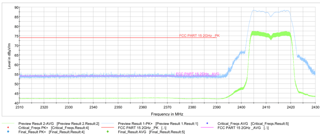
Fig.A.6.2.3 Transmitter Spurious Emission - Radiated (Power): 802.11g, ch1, 2.31 GHz - 2.43GHz
