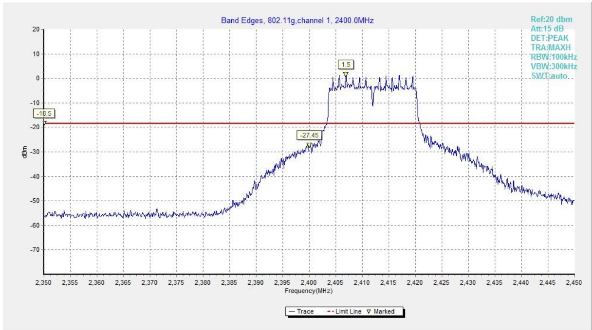
Fig.A.5.3 Band Edges (802.11g, Ch 1)
