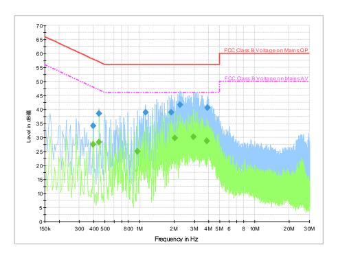
Fig A.7 Conducted Emission from 150kHz to 30MHz
