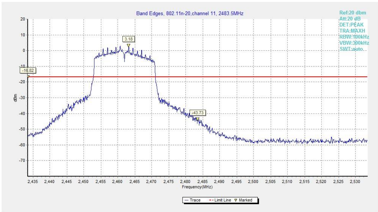
Fig.30 Band Edges (802.11n-HT20, CH 11)
