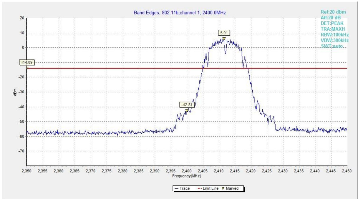
Fig.25 Band Edges (802.11b, CH 1)
