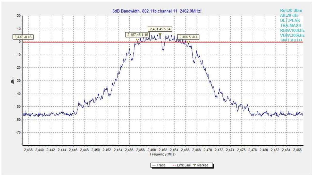
Fig.15 6dB Bandwidth (802.11b, CH 11)
