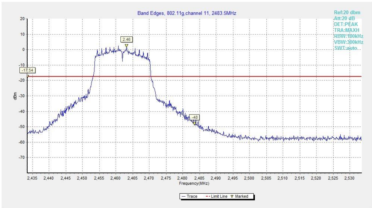
Fig.28 Band Edges (802.11g, CH 11)
