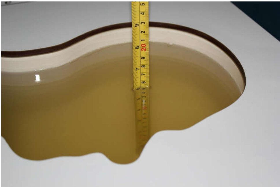
Picture 7-6: Liquid depth in the Head Phantom(2550MHz)
