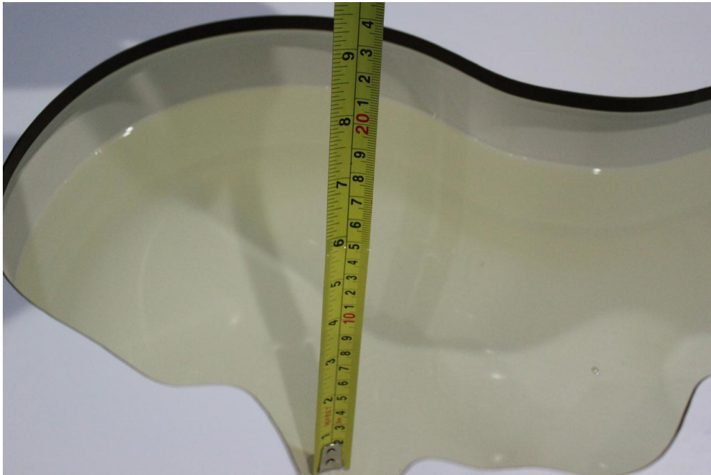
Picture 7-7: Liquid depth in the Head Phantom(5GHz)
