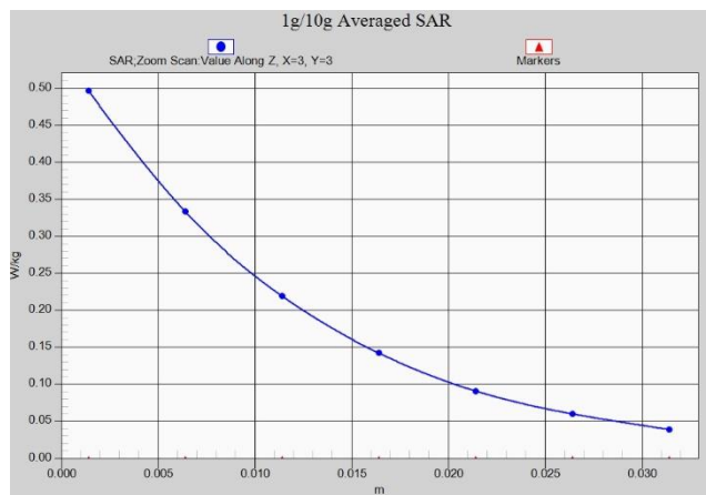
Z-Scan at power reference point (LTEB2)
