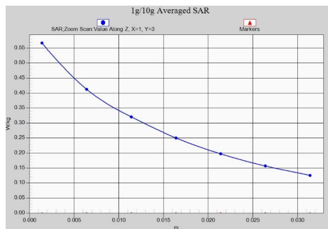
Z-Scan at power reference point (LTEB5)
