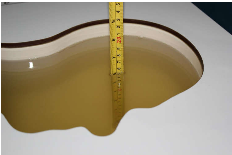
Picture 7-6: Liquid depth in the Head Phantom(2550MHz)
